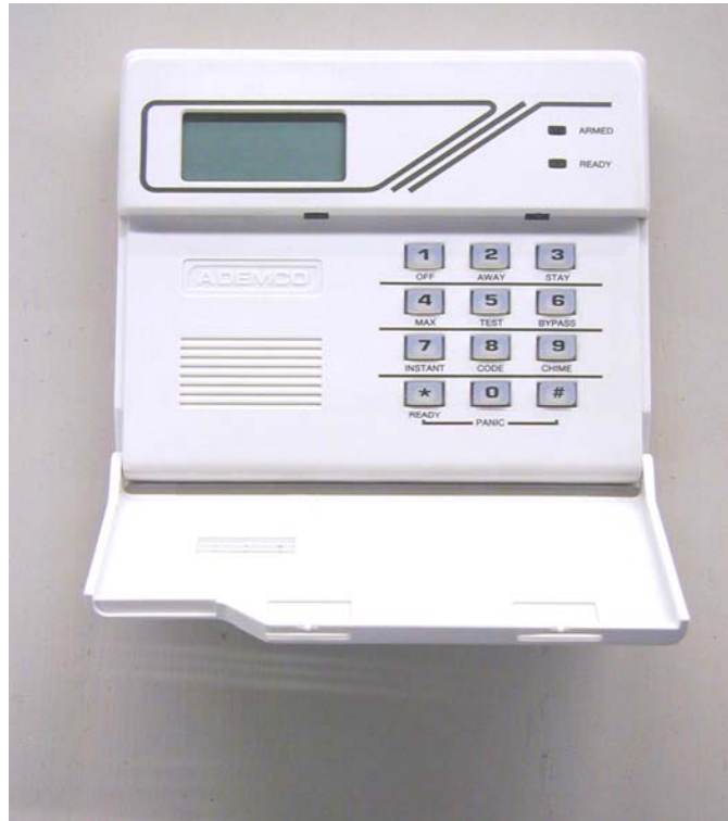
Figure 58: Intrusion Alarm Keypad
