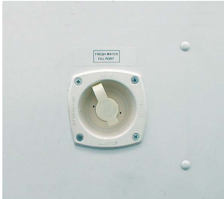
Figure 26: Humidifier Tank Fill
