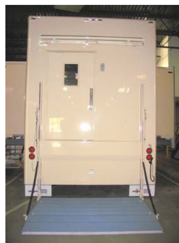
Lift Lowered without Handrails
