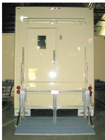
Lift Lowered with Handrails
